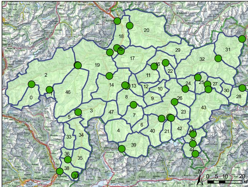
Figure 5: Division of the whole domain into 48 individual catchments, green dots representing existing gauging stations. Base map ©2009 SwissTopo.
